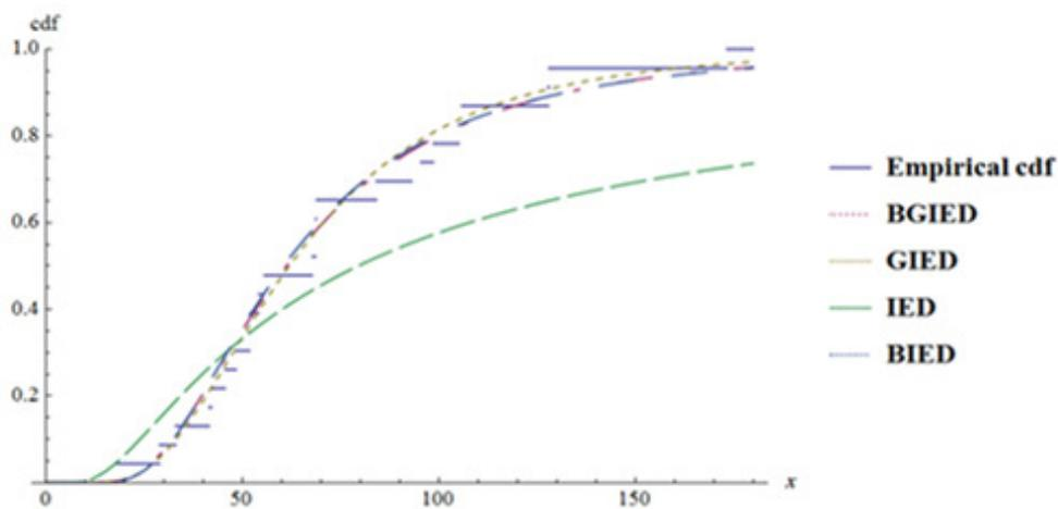
**Figure 4:** The empirical distribution and estimated cdf of the models for the ball bearing data.
